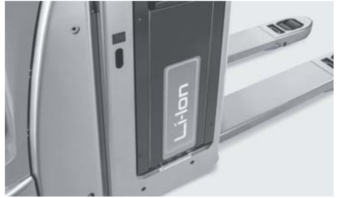
Increased operational hours thanks to fast interim charging with optional STILL Li-ion technology 2
