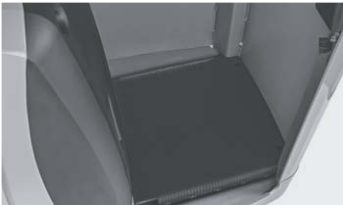
Operator comfort: cushioned stand-on platform for the driver improves ability to concentrate 3
