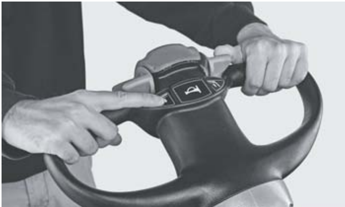
Ergonomic and intuitive operation: driving, lifting and steering processes can be controlled single-handedly by either left- or right-handed operators 1
