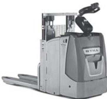
Single-handed control of all functions for right-handed as well as left-handed drivers thanks to the STILL combi-tiller
