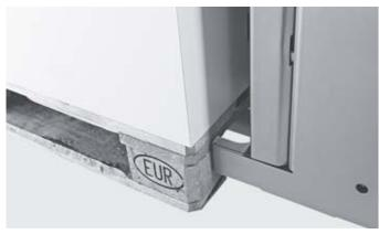
Precise double deck stacking thanks to the unique EXD 18 pallet positioner
