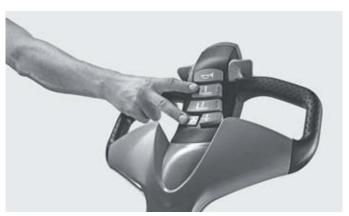
Precise handling of the EXD 18 and EXD 20: lift and lowering buttons can be haptically distinguished
