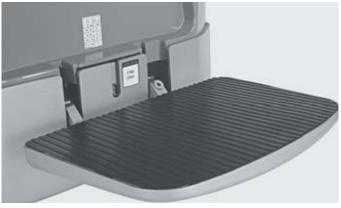
The pneumatically dampened stand-on platform ensures fatigue-free work and less strain for the driver
