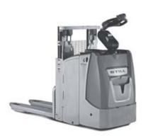
Single-handed control of all functions for right-handed as well as left-handed drivers thanks to the STILL combi-tiller
