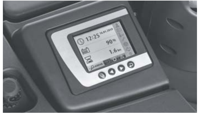
Everything in view: colour display with language-independent symbols shows all of the important functions
