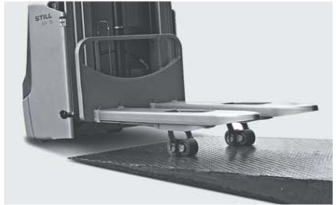
Best suited to ramps: initial lift helps the EXV drive up ramps with ease
