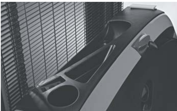
Hands free: practical storage compartments and a writing pad with built-in clipboard
