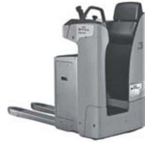
The SXH low lift pallet truck combines many economic benefits in a single truck. The SXH is the perfect solution for tough applications such as loading and unloading lorries and fast horizontal transport. It quickly moves loads of up to 2,000 kg anywhere. At full power it masters quick sprints with speeds of up to 12 km/h thanks to its powerful drive. Loads are also easily moved on gradients thanks to the optional level compensation.
