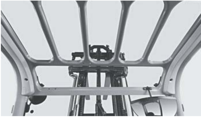
Optimum visibility thanks to narrow protective roof profiles
