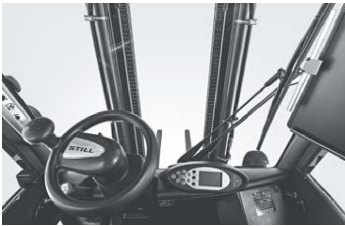
Excellent visibility to the front due to clear-view mast and low dash panel
