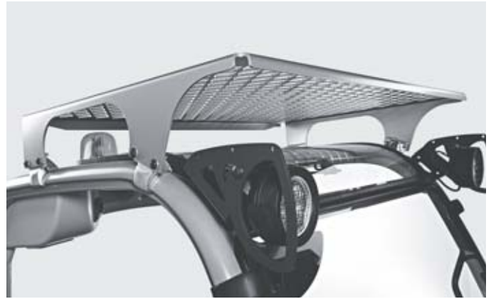
Additional protective grille roof
