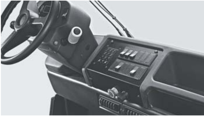
Electric parking brake and functional dashboard with compartments for documents and working materials
