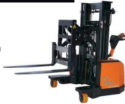
The Flexi AC NANO TW/FW electric two-way pedestrian operated stacker is perfectly suited for handling palletised goods in very narrow aisles. It has many uses in the warehousing and retail storage industries. The Flexi AC NANO is also available in optimal four-way format and is an excellent piece of equipment for long load applications in the wood, furniture, materials, sanitation, windows and doors, and the steel industry.
