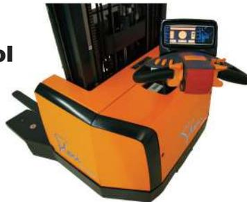
The robust fork reach system uses a hydraulic pantograph fork carriage which offers an unrivalled field of view at every lift height and more importantly the ability to pick up any design of wooden pallet either closed (ISO) or open (EURO) type.
