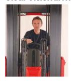
FLEXI operators have excellent visibility thanks to a standard 'Hi Vis' lift mast which has four side mounted lift cylinders. Mast tilt allows easy fork entry into pallets - even on lorries.
