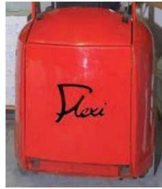
Detailed steel plate rear panel protects traction battery. Narrow 1000mm wide rear chassis allows block stacking and drive in rack operation. Handles Euro alliance pallets in 2 metre aisle to DIN I51.
