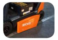
Tool-less removable side panel The side panel can be removed without the need for any tools, not even a screwdriver, saving valuable time for the operator or service technician. Thanks to the wide open hood angle, components are easily accessible for servicing.
