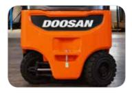
Optimised steering angle BT (3-wheel truck): 90° BX (4-wheel truck): 86°
