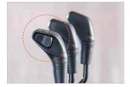
Ergonomically designed hydraulic levers with F/R switch
