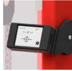
Touch screen. Log function. Possible to program e.g. several stops, turning angle, speed, rotation. Shows error messages.
